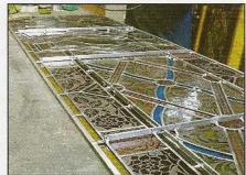
Above - The art of "box bracing" means that stained glass windows last far longer by providing vertical and horizontal support. Many shops that charge more do not provide this service.
